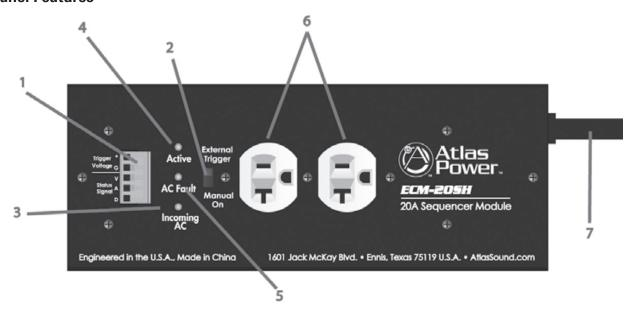
1. Trigger / Status Port Pin Identification - All signals are of low voltage and current.
