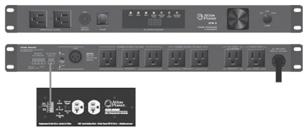
**ECM DCV Trigger** - The ECS-3 can handle 15A of current before the breaker opens. If 15A is not enough current to support your power requirements you can use the 24VDC trigger to activate an additional power outlet such as the ECM-20SH. This triggered 24VDC voltage works in conjunction with Sequence 3 timing section. Contact Atlas Sound for AC outlet options.
