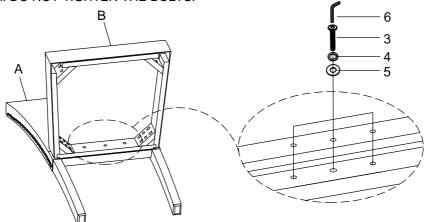
STEP 2: Place the chairback (A) on a soft and clean surface. Assemble the cushion seat (B) with the chairback (A) by using Allen Key (6) with hardware 1,4, and 5.
