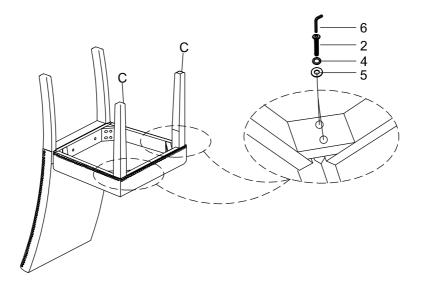
STEP 4: To level the chair, stand the chair up on a flat surface and tighten all the bolts by using Allen Key (6).
