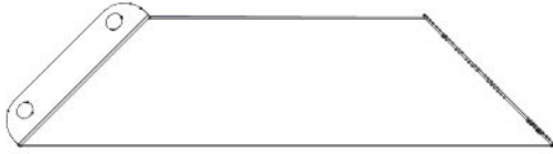
C01 CORBEL ASSEMBLY - A4M03525 (x1) 21 13/16"x5 1/4"x2 3/4" (70x134x553.5)
