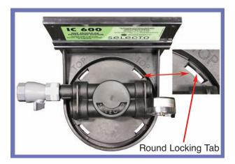
4. If leakage persists, remove cartridge by following the procedures outlined in "Step 1" of the Cartridge Changing Instructions on Page 5. Inspect the O-Ring on the top of the cartridge for damage. Replace with a new O-Ring (supplied) and lubricate well with lubricant supplied. Replace the cartridge by following the procedures outlined in "Step 2" of the Cartridge Changing Instructions on Page 5. See diagram below.
