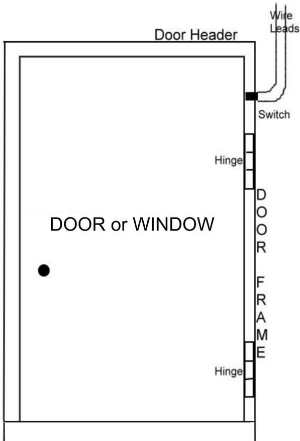
ON HINGE SIDE of door or window frame drill a 3/4" hole for the switch
