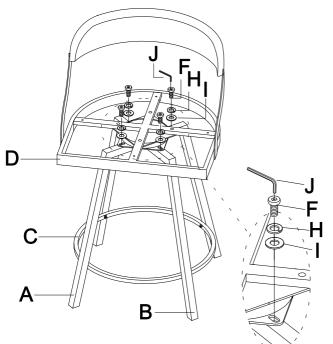
Stand the chair on an even surface and check for balance. If the chair wobbles slightly, apply downward pressure on the uneven leg and tighten the bolts to correct the imbalance. Once the chair is balanced, apply downward pressure evenly in the center of the chair and tighten all bolts, being careful not to over-tighten beyond the hole depth. 3 Attach Seat Cushion (E) to Back with Swivel Plate (D) using Screw (K) with a screwdriver (not provided).
