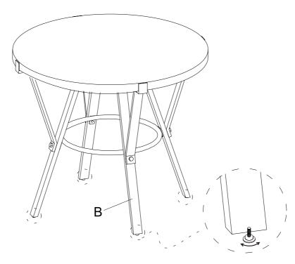
Adjust the height of the pre-installed levelers to achieve balance.
