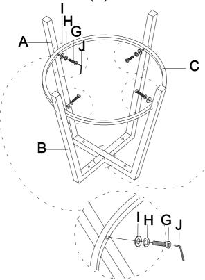
Take the Allen Wrench and turn the bolts until the legs are secured. DO NOT TIGHTEN THE BOLTS COMPLETELY. Stop when you feel you are adding force to tighten the bolt.
