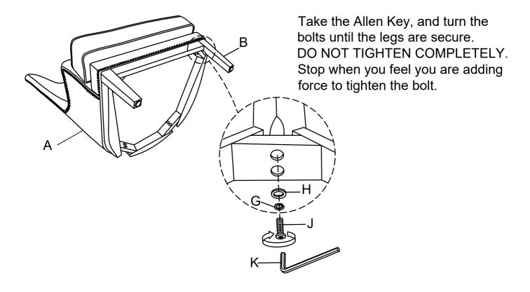
Then attach the Back Leg (C) to the Chair Body (A) using the Bolt (I), Lock Washer (G), Flat Washer (H) in both holes of Back Leg (C) and Chair Body (A), turn the Allen Key (K) in Bolt (I).
