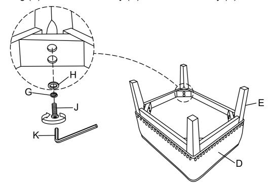
Put the Chair Body (A) on a smooth flat surface, attach the Front Leg (B) to the Chair Body (A) using the Bolt (J), Lock Washer (G), Flat Washer (H) in both holes of Front Leg (B) and Chair Body (A), turn the Allen Key (K) in Bolt (J).
