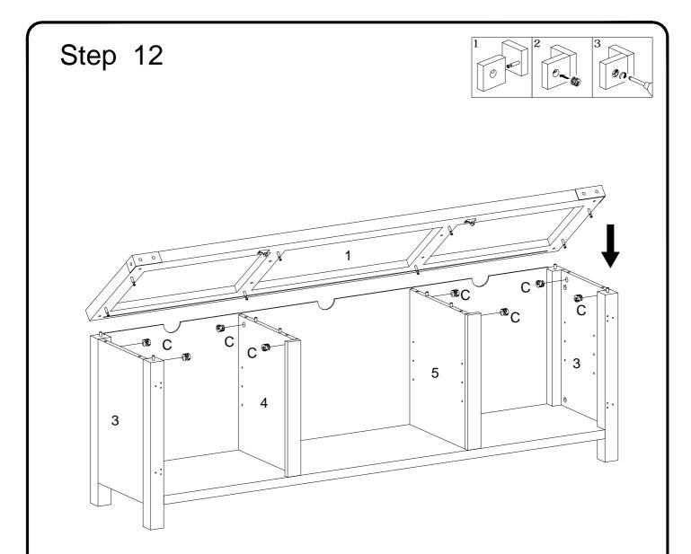
Insert part (1) into part (3,4,5), then insert and secure cam lock (C) to part (3,4,5).
