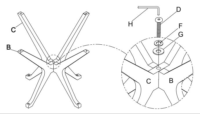
Attached Leg Up(B) and Leg Down(C) to the Table Top(A). Use Allen Bolt(E) Lock Washer(F) and Flat Washer(G) on holes of Table Top(A). Turn the Allen Key(H) in Allen Bolt(E).
