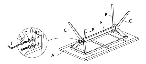
With assistance from your adult partners, turn the Dining Table right way up. Adjust the Pre-installed Levelers on the bottom of Left Leg (B) and Right Leg (C) until the Dining Table is level with the ground.
