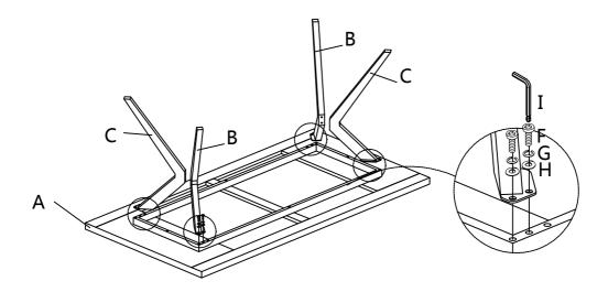
Attach Iron (D) to Left Leg (B) and Right Leg (C) using Bolt (F), Flat Washer (H) with Allen Key (I).
