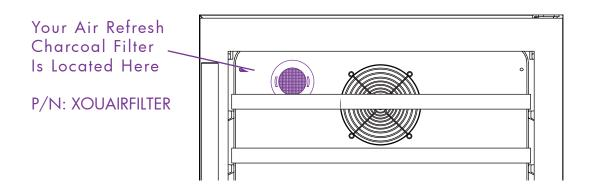
Rotate the filter 1/4 turn to unlock
