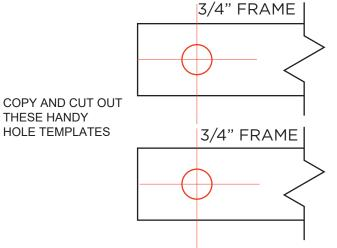
TO ACCOMMODATE THE HINGE PINS ON THE HINGE SIDE OF THE PANEL Drill a hole at least 5/16" in diameter and 1" deep into the top and bottom of the frame in the location shown.
