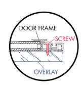
7 Using the (10) ST4-30 self-tapping screws supplied securely fasten each frame to the door. Do not over tighten as screws may strip out. WARNING: Screws are sized for 3/4" panel, DO NOT USE these screws for thinner panels.
