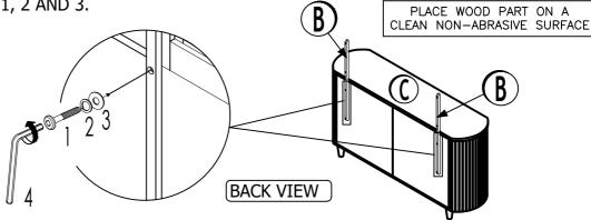
STEP 2: Assemble the Mirror Support (B) with the Mirror (A) by using Allen Key (4) with hardware 1, 2 and 3.
