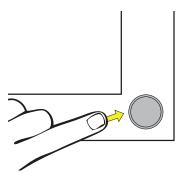
**4.** A quick touch and release will turn the lights on/off. Touch and hold with increase or decrease the light output.
