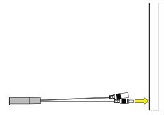
2. Run wires through hole and insert touch dimmer switch into hole.
