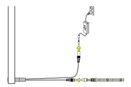
3. Insert male plug from power supply into female plug on touch dimmer switch. Insert male plug on touch dimmer switch into a female barrel connector that is wired to the lighting. NOTE: The female barrel connector can be borrowed from a plug-in power supply.
