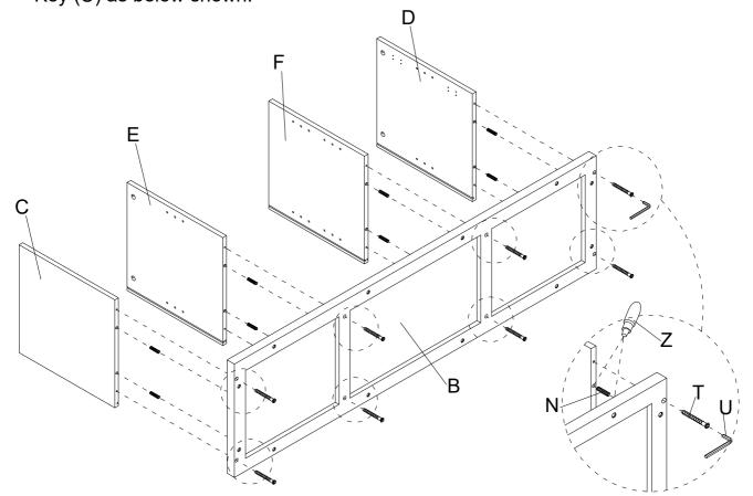
Insert Side Back Panel (J) & Middle Back Panel (K) to pre-assembled Side Panel - L (C), Side Panel - R (D), Middle Panel - L (E) & Middle Panel - R (F) and Bottom Panel (B) as below shown.
