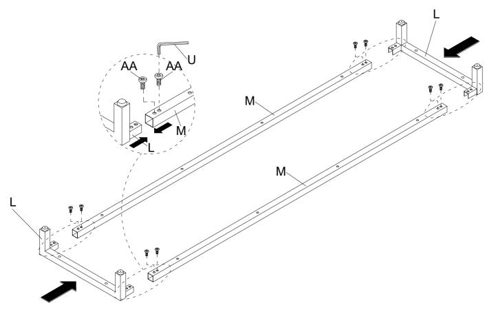
Attach pre-assembled Leg Frame (L) and Stretcher Bar (M) to Bottom Panel (B), using Bolt (AB) by Allen Key (U) as below shown.
