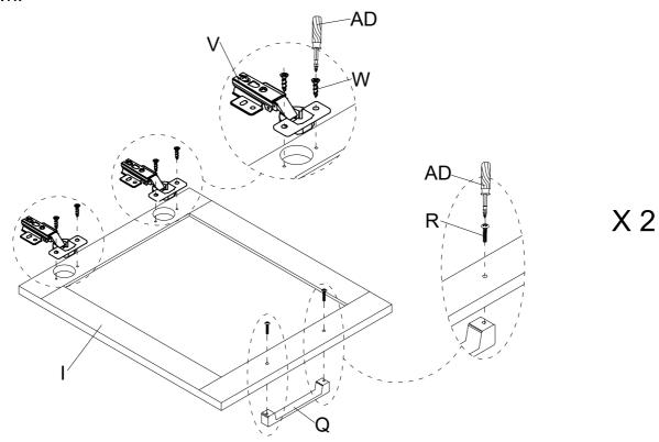
Assemble Door Panel (I) to Side Panel - L (C) and Side Panel - R (D) through Hinge (V), using Screw (W) by Screwdriver (AD) as below shown.
