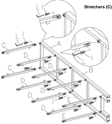
Stretchers (C)'s gaps should face upward.
