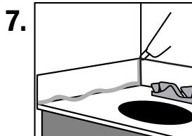
Apply 100% silicone to the seam where the side splash touches the cultured marble (indicated by gray line). Apply "kitchen & bathroom caulk" to the top edge of the side splash that touches the wall (if installing a side splash).
