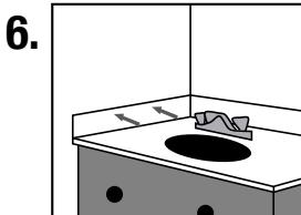
Carefully push the side splash in place, making sure you firmly press it against the wall. (If installing a side splash)
