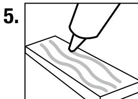
Use "Liquid Nail" or "PL Adhesive". Apply a generous amount to the back of the side splash (if installing a side splash).
