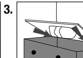
Apply adhesive to the back of the backsplash. Clean off any excess silicone and place the vanity on the cabinet, back first.
