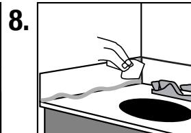
With a caulk edging tool, run it across the seams to clear away excess silicone & caulk (this technique will leave a clean line of silicone & caulk over the seams). (If installing a side splash)
