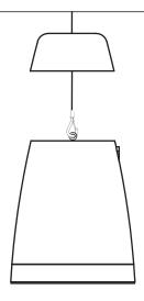
5. Connect the safety hook to the hole hanger attached to the speaker as shown.
