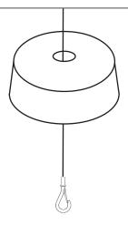
3. Thread the cable that's attached to the mounting structure through the hole of the back cover and attach the saftey hook.
