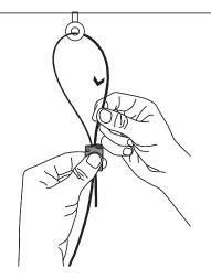
4. Press the button on the gripple and slide the cable through to the desired height to adjust speaker height.
