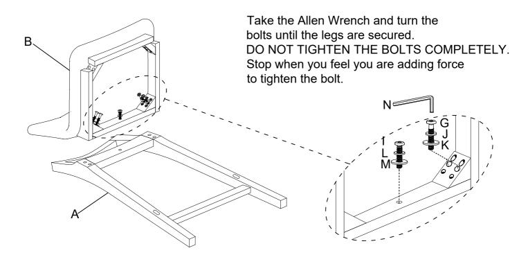
Attach Front Leg (C & D) to Seat (B) using Bolt (H), Spring Washer (J) and Flat Washer (K) with Allen Wrench (N). Half tighten all the bolts in this step.
