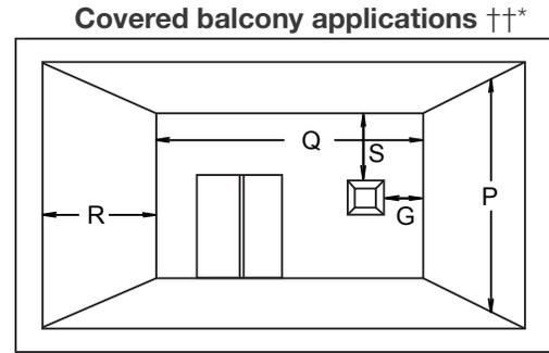
$Q_{MIN} = 3 \text{ feet (0.9m)}$      $R_{MAX} = 2 \times Q_{ACTUAL}$      $R_{MAX} \leq 15 \text{ feet (4.6m)}$
