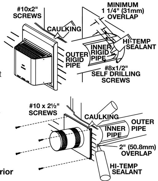
**The air terminal mounting plate may be recessed into the exterior wall or siding no greater than the depth of the return flange.**
