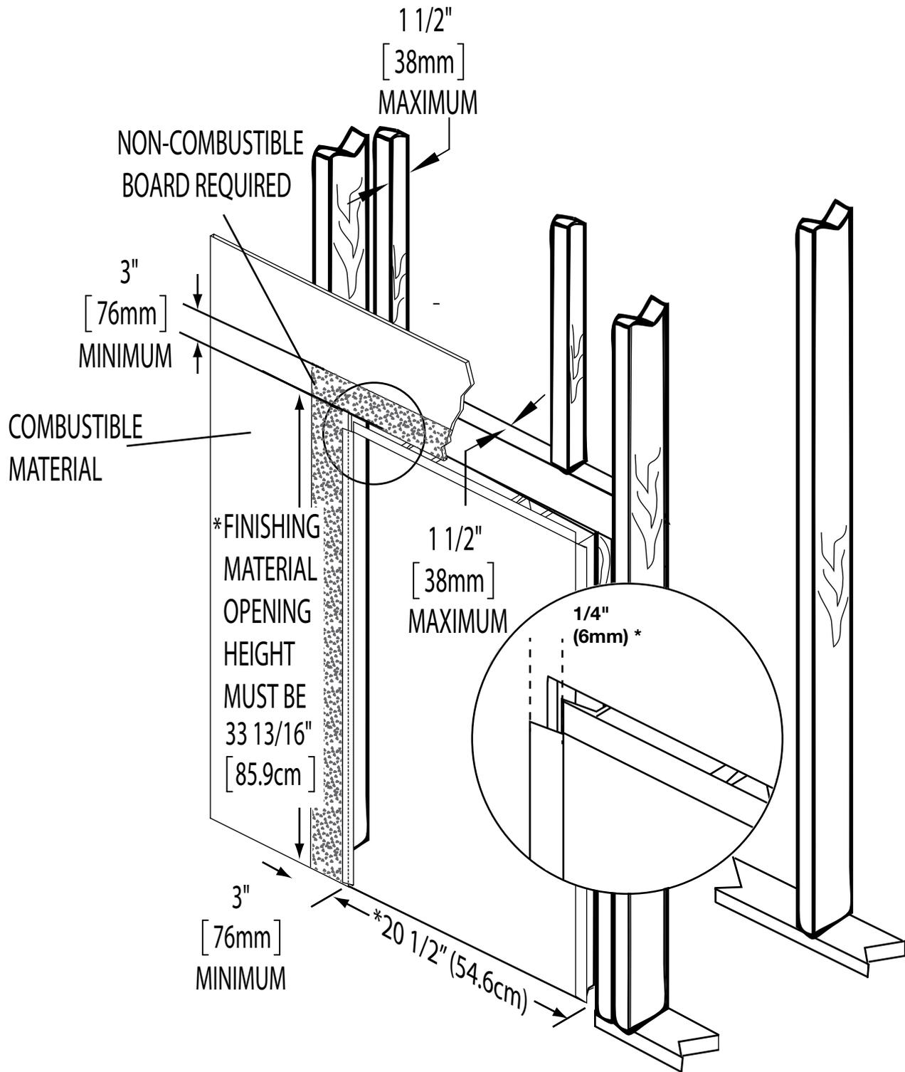
\* Finishing material **MUST NEVER** be installed behind the finishing flange.
