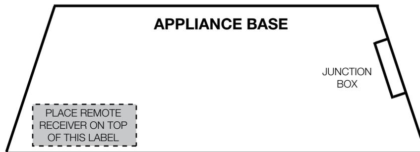
Position the remote receiver in the valve compartment box. Ensure the receiver is on top of the placement label, if equipped.
