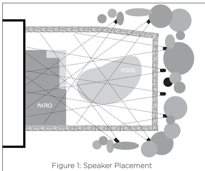
Use care to select satellite locations that are equally distant from the main listening area. When possible, use high and low locations to centralize the acoustic stage (see Figure 2).
