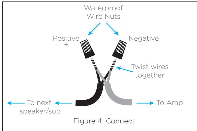
**IMPORTANT: Be sure not to let any stray '+' and '-' strands touch each other. Touching strands can cause a short-circuit that could damage your amplifier and degrade sound quality.**
