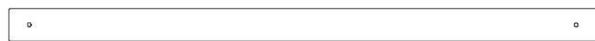
M02 | RAIL MURAL - W4L13943 (x1) | 5/8 po x 3 3/8 po x 61 1/4 po (16 x 86 x 1 556)
