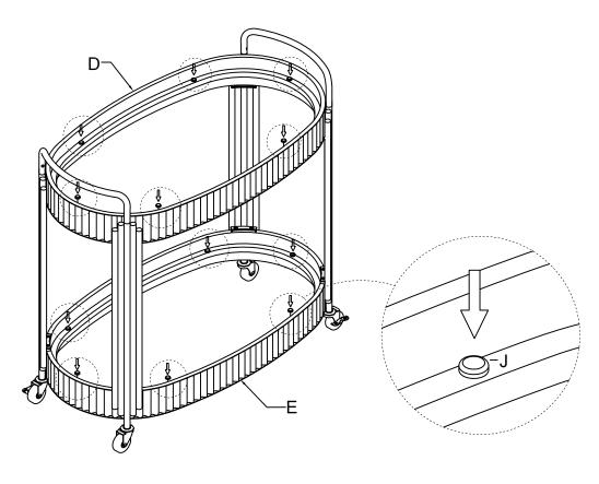
Place the Glass (F) to the Bottom Frame (E) as shown.
