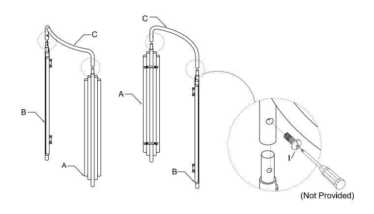
2 Attach the Leg (A & B) to the Upper Frame (D) using Bolt (I) with a screwdriver (not provided).
