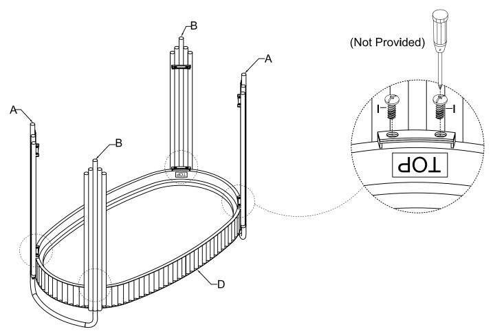
Stand the assembly unit upright. Attach the Bottom Frame (E) to the Leg (A & B) using Bolt (I) with a screwdriver (not provided).
