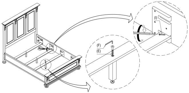
IF THE BED SUPPORTS ARE NOT LEVEL WITH THE FLOOR, ADJUST THE ADJUSTABLE LEVELERS FOUND ON THE BOTTOM OF THE LEG SUPPORTS.
