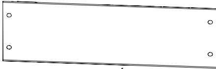
B04 FAISCEAU LATÉRAL - A4M02019 (x1) 1 7/16"x5 1/4"x18 7/8" (36x134x480)
