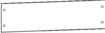
B11 FAISCEAU LATÉRAL - A4M02106 (x1) 1 7/16"x5 1/4"x18 7/8" (36x134x480)
