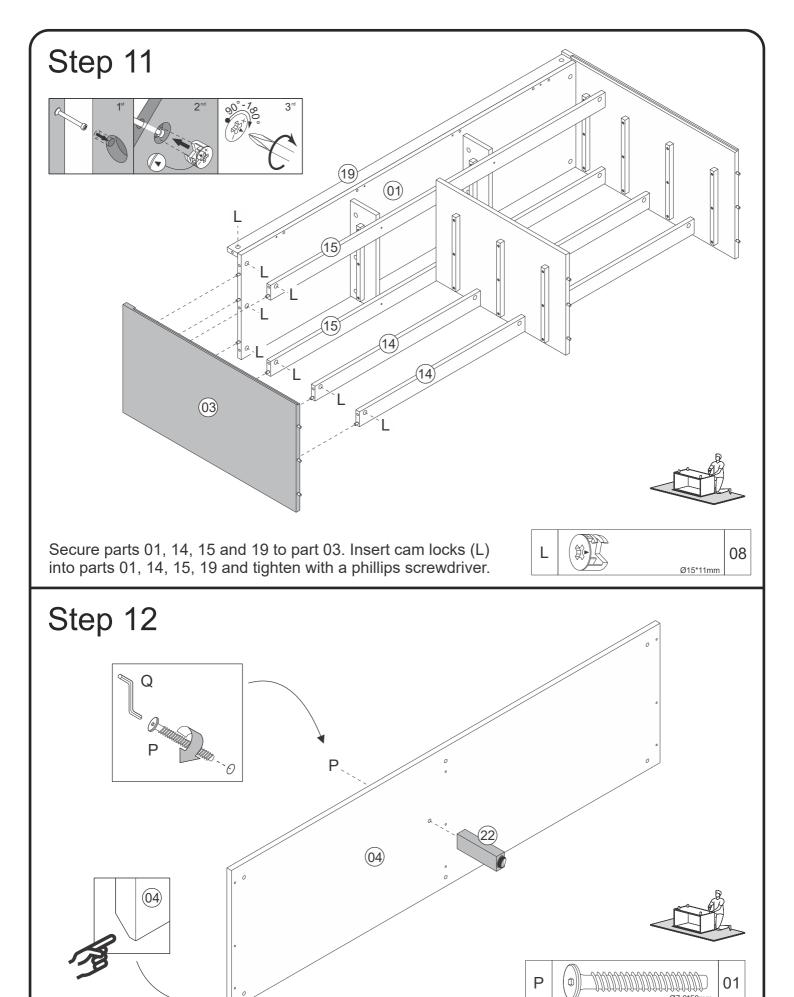
Attach part 22 to part 04 with bolt (P) and hex key (Q).
