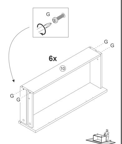
Insert parts 09 and 10 between parts 05, 06 and 07. Secure part 10 with screw (G) and phillips screwdriver.
