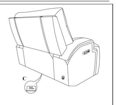
Step 5: Connect the transformer (C) to the power socket on Seat (A).
