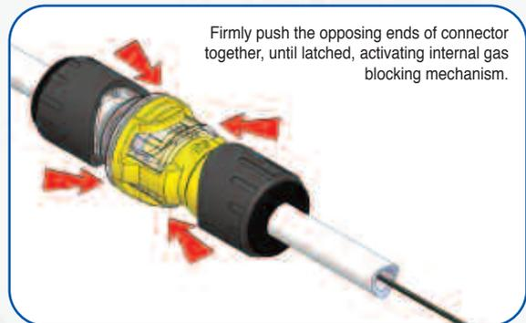
Firmly push the opposing ends of connector together, until latched, activating internal gas blocking mechanism.
