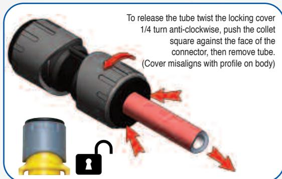
To release the tube twist the locking cover 1/4 turn anti-clockwise, push the collet square against the face of the connector, then remove tube. (Cover misaligns with profile on body)
