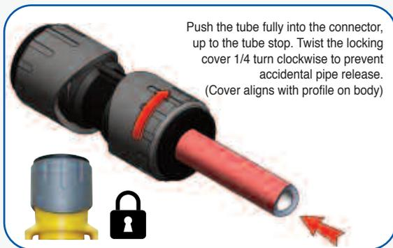
Push the tube fully into the connector, up to the tube stop. Twist the locking cover 1/4 turn clockwise to prevent accidental pipe release. (Cover aligns with profile on body)
