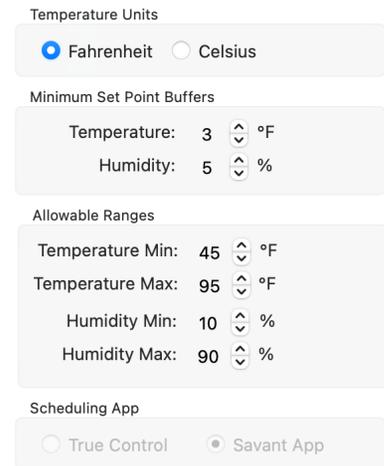
A configuration panel for HVAC settings. It includes sections for 'Temperature Units' (Fahrenheit selected), 'Minimum Set Point Buffers' (Temperature: 3 °F, Humidity: 5 %), 'Allowable Ranges' (Temperature Min: 45 °F, Temperature Max: 95 °F, Humidity Min: 10 %, Humidity Max: 90 %), and 'Scheduling App' (Savant App selected).
