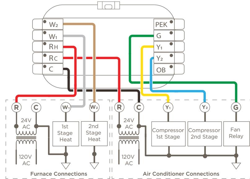
**i** **HELPFUL!** In both diagrams above, the power source from the cooling system powers the thermostat.
