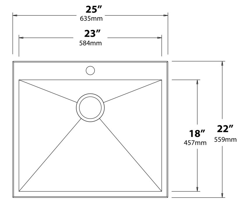
**NOTE:** Cutout template is provided as a guide **ONLY** and must be checked against actual sink to verify correct fit.
