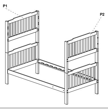
Attach the top back side rail (2 holes) marked (P6) and top front side rail (3 holes) (P7) with side panel (P1) and side panel (P2) by using screws (H1) and helix (H2) but do not fully tighten screws by allen key (H8).
