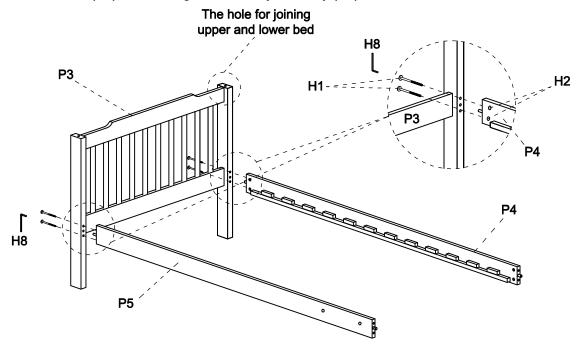
Attach the bottom back side rail (P4) and bottom front side rail (P5) join them to side panel (P3) and tighten screws by allen key (H8) and put 4 pcs metal dowels (H5) into the holes joining bed.
