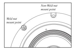
3.) Using 4 pcs -  $#10 \times .75$  in sheet metal screw, attaching the baffle / driver to the back can. Be sure to match the mouting holes <u>without</u> weld nuts to clip nuts on back can.
