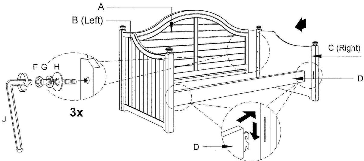
**3** Place Slats (E) to the Back Panel (A) and Front Rail (D). Secure the Slats (E) with Spring Washer (G) and JCBC Bolt (F) and tighten using Allen Key (J) & CSK Screw (I) following the diagram below.
