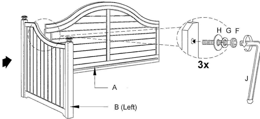
**2** Attached Side Frame (C) (Right) to Back Panel (A) by inserting JCBC Bolt (F) with Spring Washer (G) and Flat Washer (H) into provided holes. Do not tighten the bolts. Insert Front Rail (D) to Side Frame (B) (Left). Repeat the same process to Side Frame (C) (Right) . Then tighten all the bolts using Allen Key (J).
