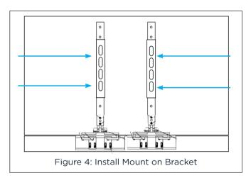
5. Tighten the bracket arm screws and the provided pinch tab screws. Loosen pinch tab screws. Slide pinch tab down into soundbar channel. Tighten pinch tabs, then tighten the bracket arm screws.
