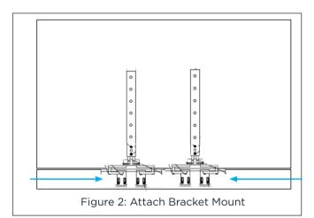
3. Loosen 10-32 Hex flathead screws on the VESA bracket and extend to match the TV's VESA hole pattern.
