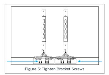
6. Tighten 10-32 Hex flathead screws on the VESA bracket to lock the bracket into position.
