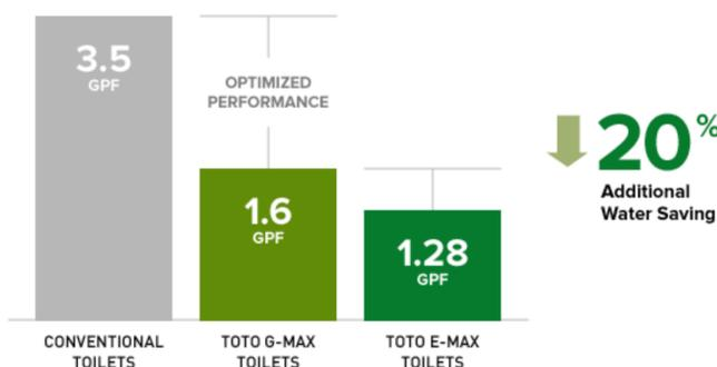
Utilizing the same proven engineering as our legendary 1.6 GPF G-Max flushing system, the 1.28 GPF E-Max reinforces TOTO's performance reputation while offering an additional water savings of 20%.
