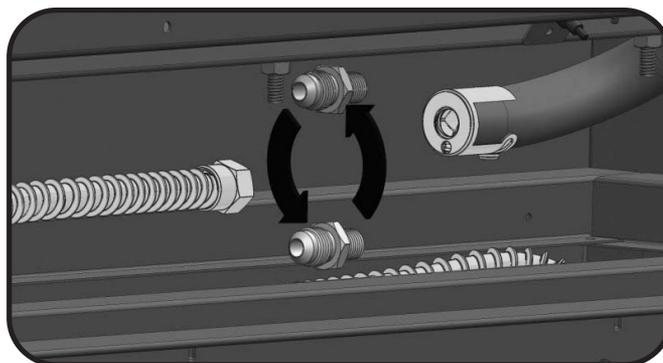
6. Replace the natural gas orifice with the LP (Propane) orifice supplied.
