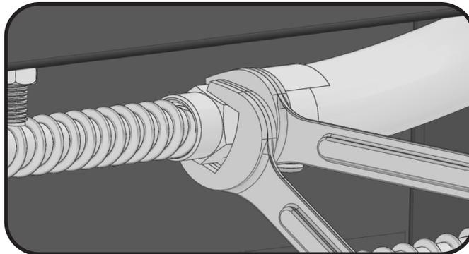
5. Unscrew the natural gas orifice from the inside of the burner as illustrated.
