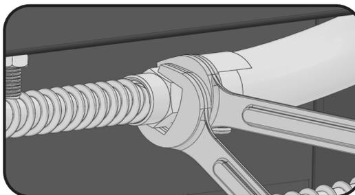
Once the glass tray is removed from the fireplace flip the glass tray upside down and remove the nuts from the bottom of the burner.
