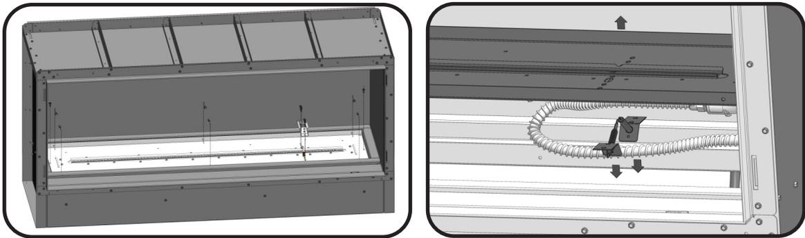
4. Disconnect the stainless steel flex connector from the orifice using (2) wrenches.
