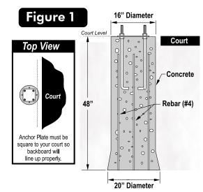
Note: The bottom four nuts will be forever embedded in concrete.
