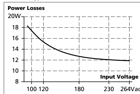
Fig. 9-4 Losses vs. input voltage at 24V, 10A, typ.
