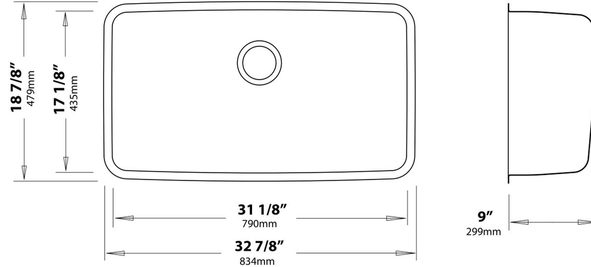
**NOTE:** Cutout template is provided as a guide **ONLY** and must be checked against actual sink to verify correct fit.
