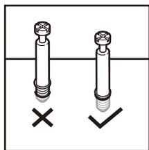
1. Screw cam bolt in completely.
