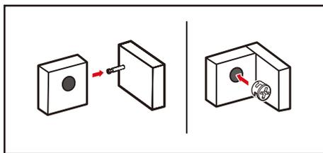
2. Insert cam bolt and cam lock into designated holes.
