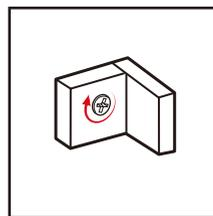
3. Screw cam lock clockwise to secure cam bolt.
