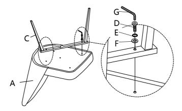
Attach Lower Leg Frame (B) to Upper Leg Frame (C) and Seat and Back (A) using Bolt (D), Spring Washer (E), Flat Washer (F) with Allen Key (G).
