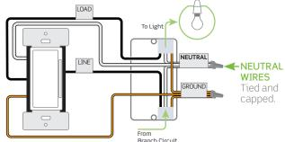
Quick tip: Check each individual location as some may have a Neutral wire and others may not. It is most common that a Neutral wire is missing in a wallbox where there is no bundle. Scan the code below for more information on how to identify a Neutral wire.
