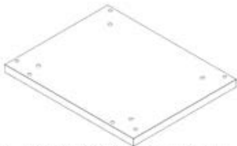
T4 PIZZA OVEN CABINET MARBLE PANEL L - A4M03068 (x1) 1 1/4"x19 5/16"x24 1/8" (32x490x612)
