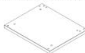
T5 PIZZA OVEN CABINET MARBLE PANEL R - A4M03069 (x1) 1 1/4"x20"x24 1/8" (32x508x612)
