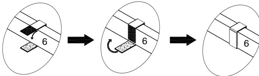
Place part (5) as per diagram , then tighten the Velcro to part (6) as per diagram.
