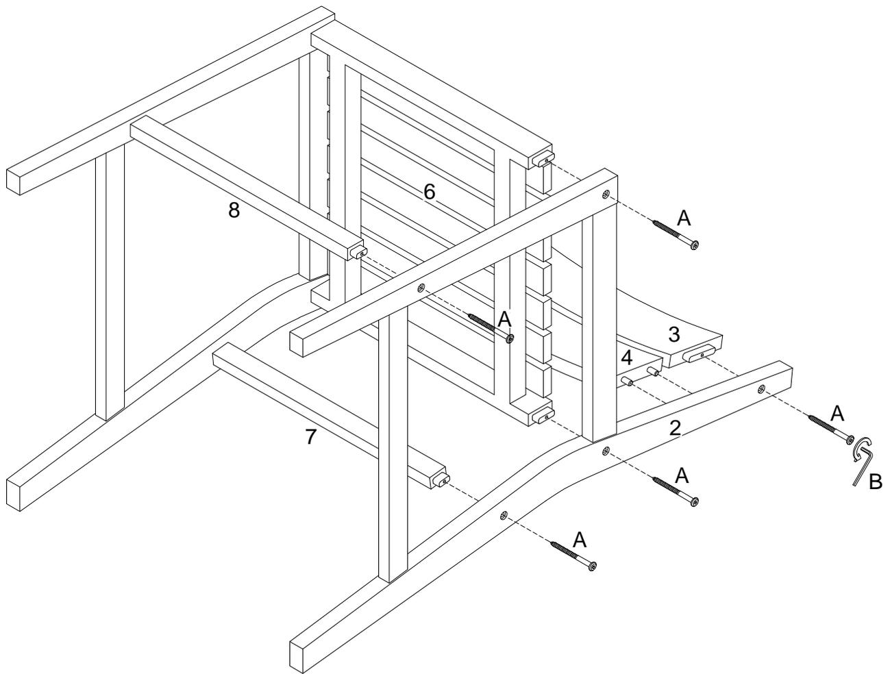
Using bolt (A) attach part (2) to parts (3,6,7,8) with hex key (B) ,attach part (4) to part (2) as per diagram .
