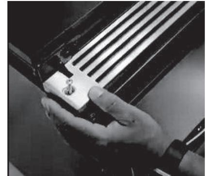
2. Remove the three screws holding the lower hinge in place.
