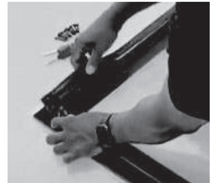
4. Starting at one corner, gently pull the rubber door gasket out
