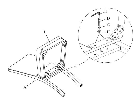
Attach Seat Cushion (B) to Chair Back (A) by securing Flat Washer (H), Lock Washer (G), Allen Bolt (E) and Allen Key (I) onto corners. Do not over-tighten.
