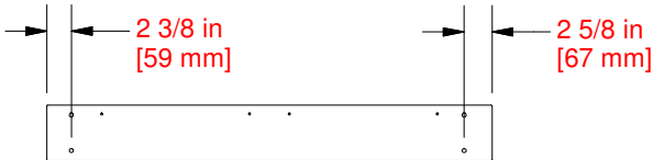
G2 GROUND BOARD - W4L17641 (x1) 1"x5 1/4"x42 1/4" (24x134x1072)
