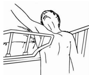
Entrapment between the end of the rail and the side edge of the head board or foot board
