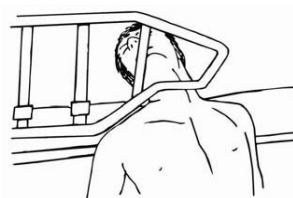
Entrapment between split bed rails
