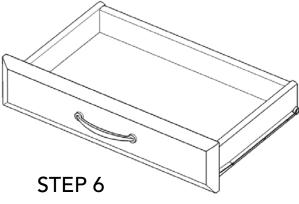
Attach Drawer Front (M1) and Drawer Back (M2) to Drawer Side (M3) with Wood Screws (long).
