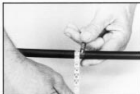
FIGURE 4 – WRAP CABLE MEA-SURE TAPE AROUND CABLE
