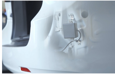
Radar Sensors Install behind plastic bumpers
